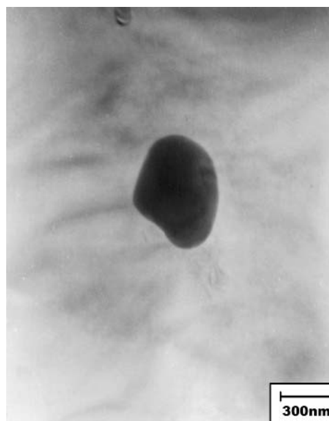
Fig. 7 AlFeSi particle in alloy 6060 (by TEM)
